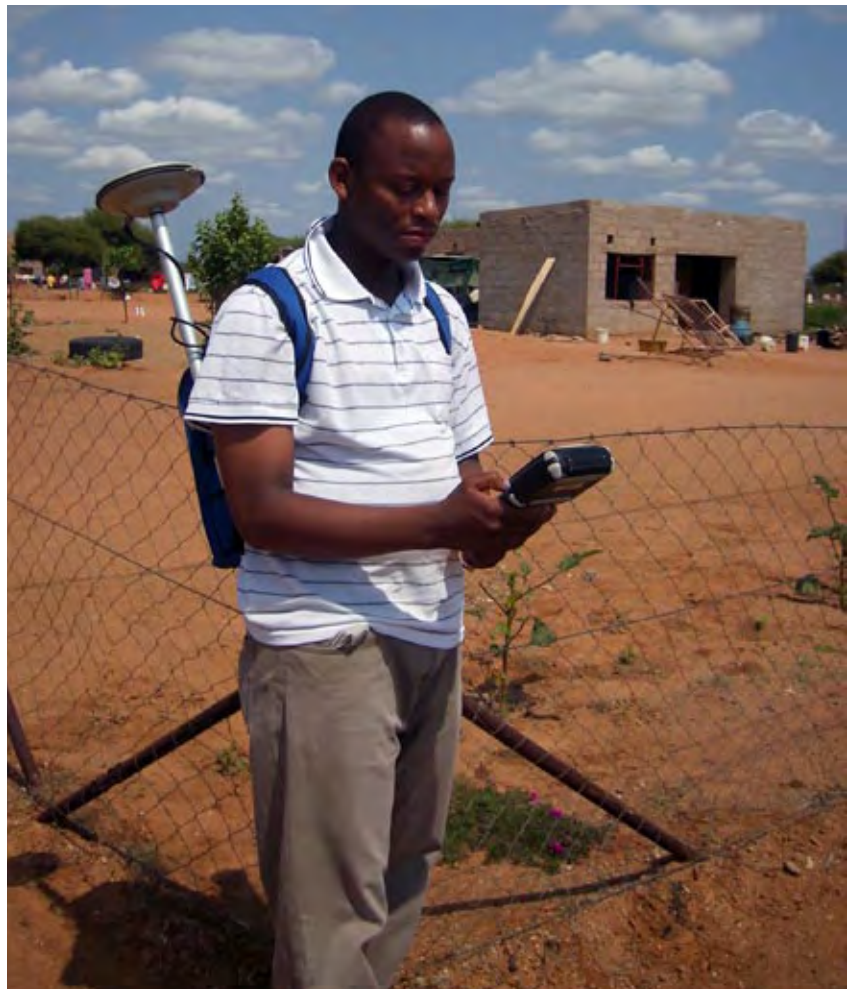
GPS technology can help survey plots to sub-metre accuracy
